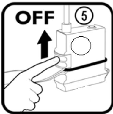
Fig 5 - Slide the side arming switch UP by lifting the rubber restrainer 'O' ring down and over the side switch and ensure the 'O' ring sits back in the gap below the side switch.
